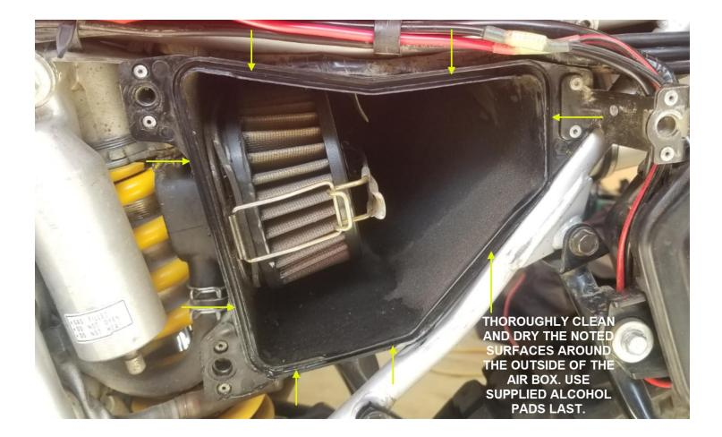
Start to peel off the backing form the supplied adhesive-backed foam tape. Install the foam tape around the outside of the air box as shown, covering the OEM rubber gasket. This will create an air seal between the air box and side panel. The foam gasket will be too long. Trim the excess as needed.
