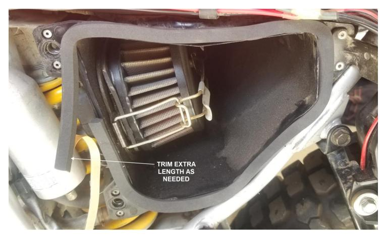
3. Press firmly all around the foam gasket to ensure it is well adhered.
