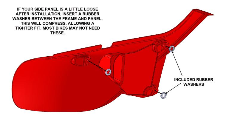
5. Some bikes are a little different from others, and one or more Dzus location might be a little loose after installation We include 3 rubber washers that can be installed between the side panel and frame if needed, to take up any extra space and prevent rattling.
