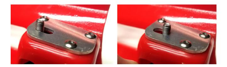
2. Install supplied aluminum studs. Adjust location as needed then apply threadlocker. Install side panel using your old bolt.
