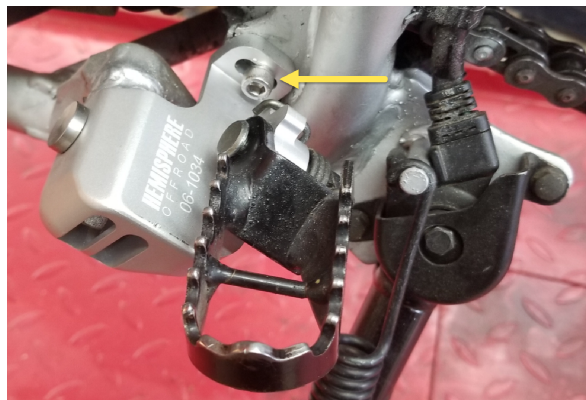
REMOVE THE STOCK SCREW FROM THIS LOCATION. REPLACE WITH SUPPLIED LONGER SCREW
