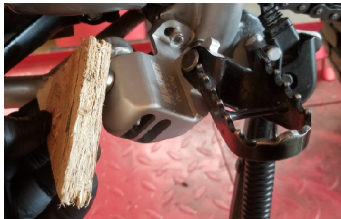
USE A PIECE OF WOOD TO PROTECT THE SURFACE IF YOU NEED TO TAP THE PIN IN WITH A HAMMER.
