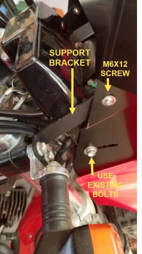
LOOSELY INSTALL THE STOCK MOUNTING BOLTS THROUGH THE CURVED SLOTS, INTO THE FRAME.
